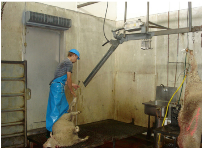
Photograph 4. Lifting the shackled smallstock carcass using the rail lifter.
