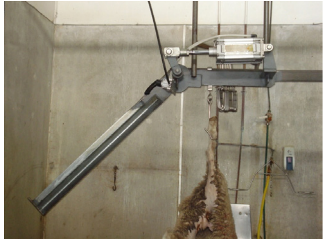
Photograph 3. Detail of the smallstock carcass lifter installation.
