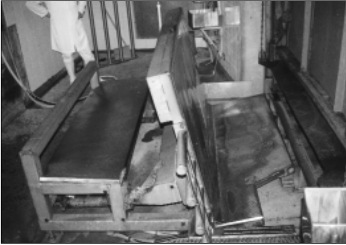
Photograph 1. The landing cradle in the lowered position.
