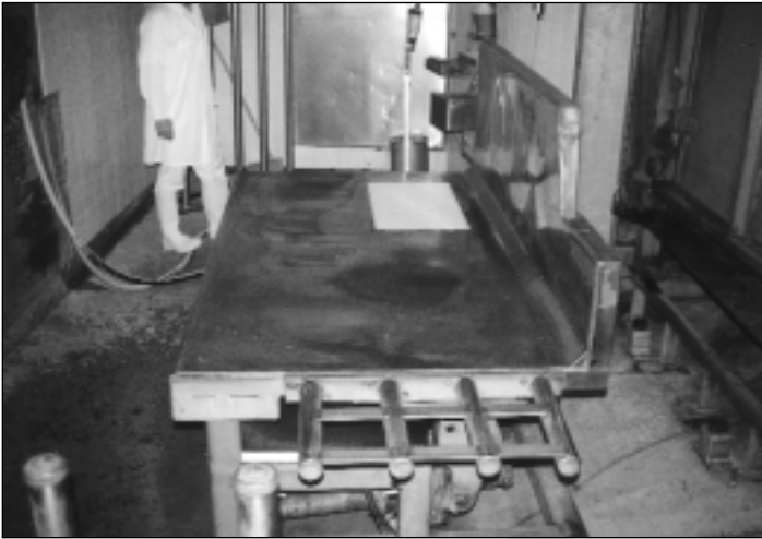
Photograph 2. The landing cradle in the raised position.
