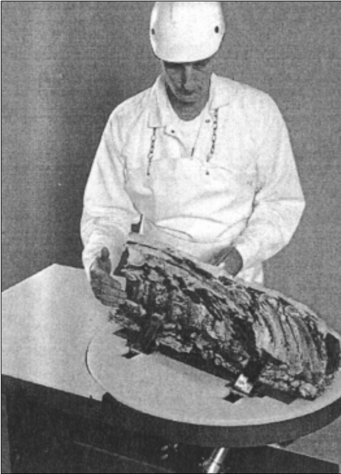
Photograph 4. Rotation of the mounting plate about the horizontal axis.
