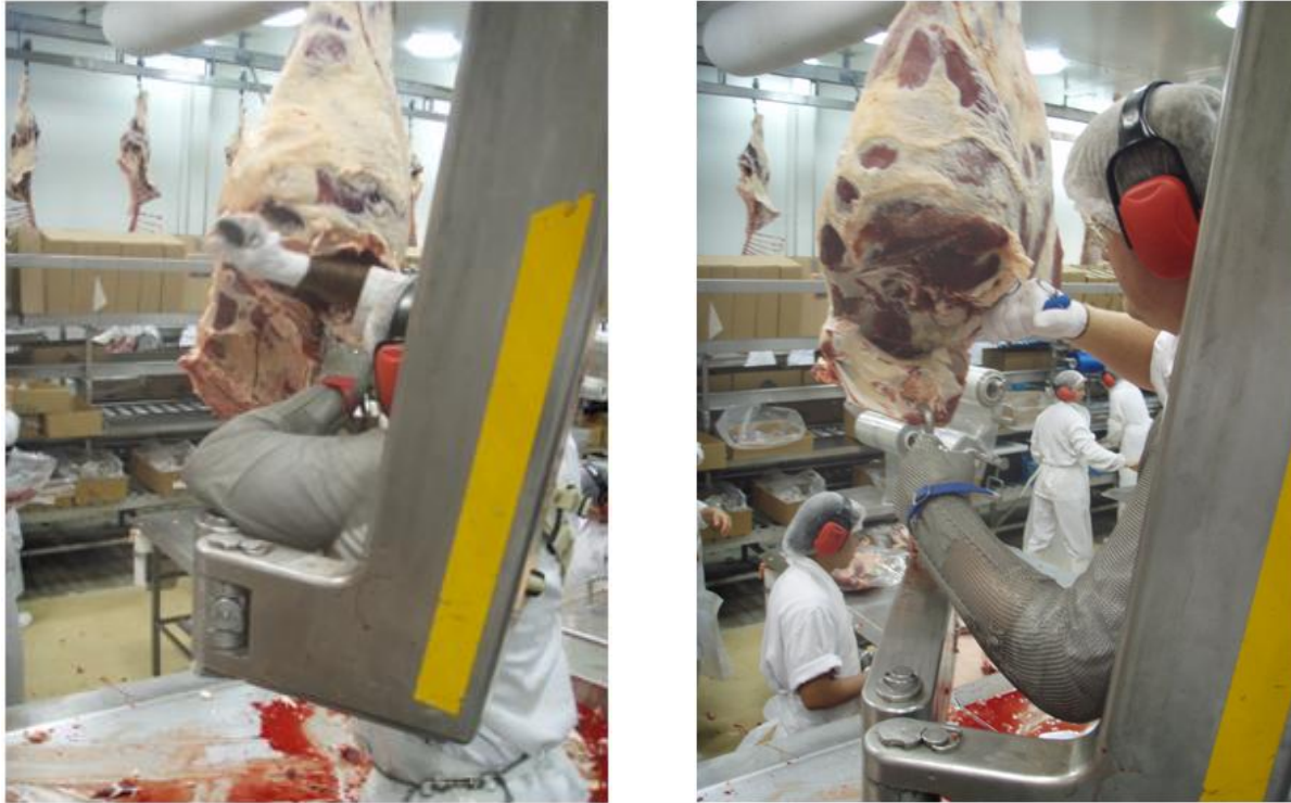
Figure 1: RTL system in operation – removal of aitch bone from butt
