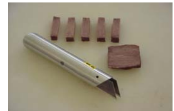
Figure 2. Prepared tenderometer samples and modified knife for accurate cutting
