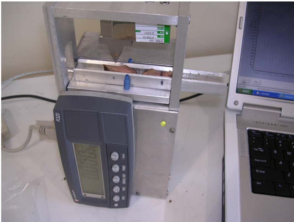
Figure 9. The G2 Tenderometer provides a convenient method for the objective measurement of meat tenderness by direct streaming of force-time data to attached PC and instrument display.
