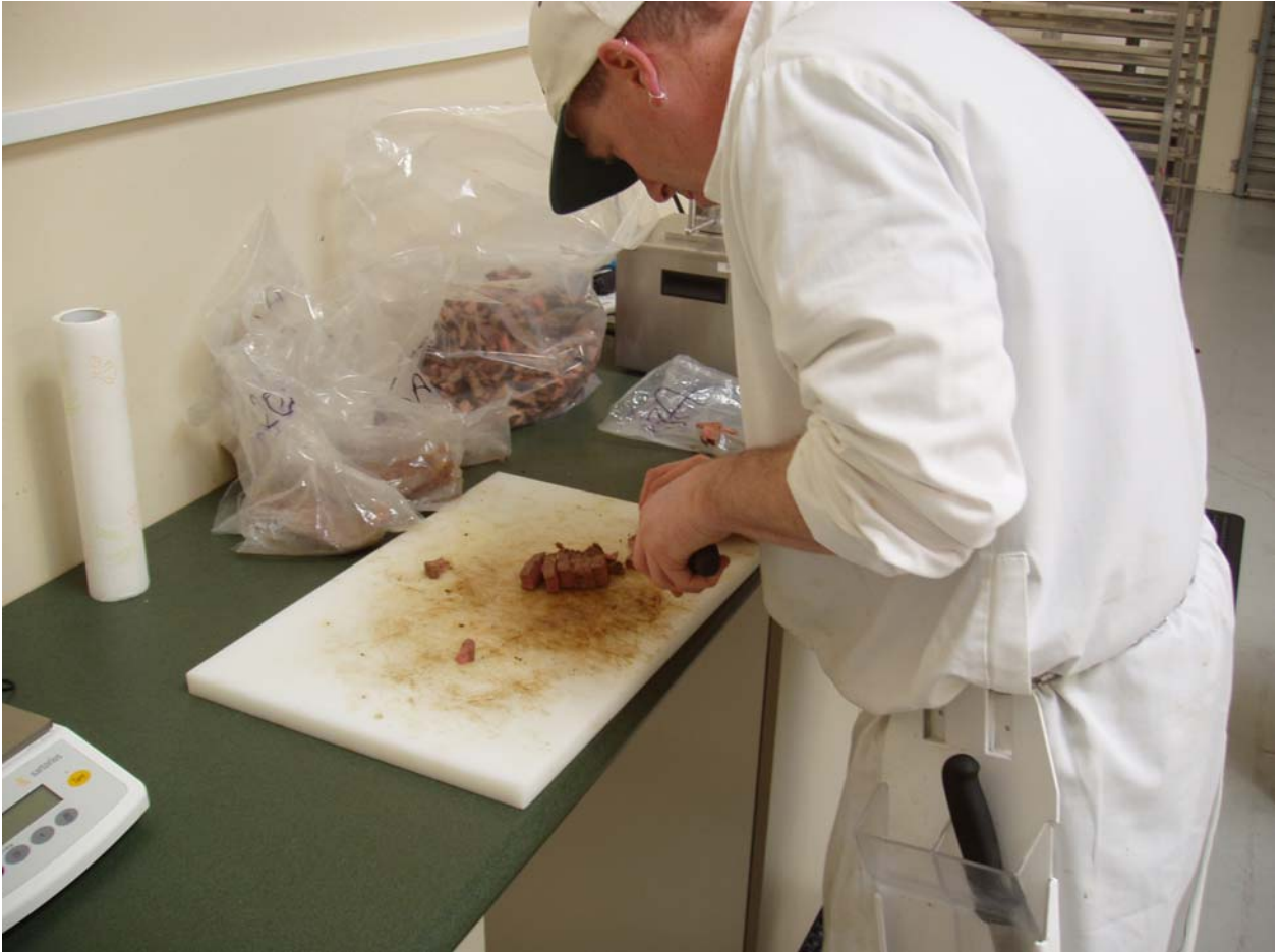
Figure 13. Meticulous preparation of specimen bites to prescribed dimensions with consistent alignment of muscle fibers bears great importance in maintaining uniformity of samples to allow useful comparison of tenderness measurements.
