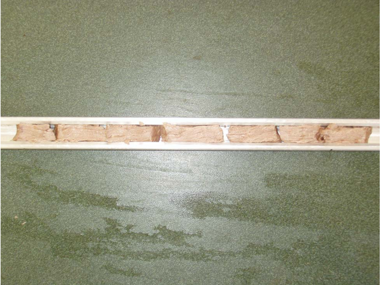
Figure 14. Meat specimens are prepared into 'bites' with cross section dimensions 10mm by 10mm and up to 50 mm long with all muscle fibers oriented in the longitudinal direction. 'Bites' are confined within an aluminium loading tray which is projected upward to the static load cell and shear/compression attachment.
