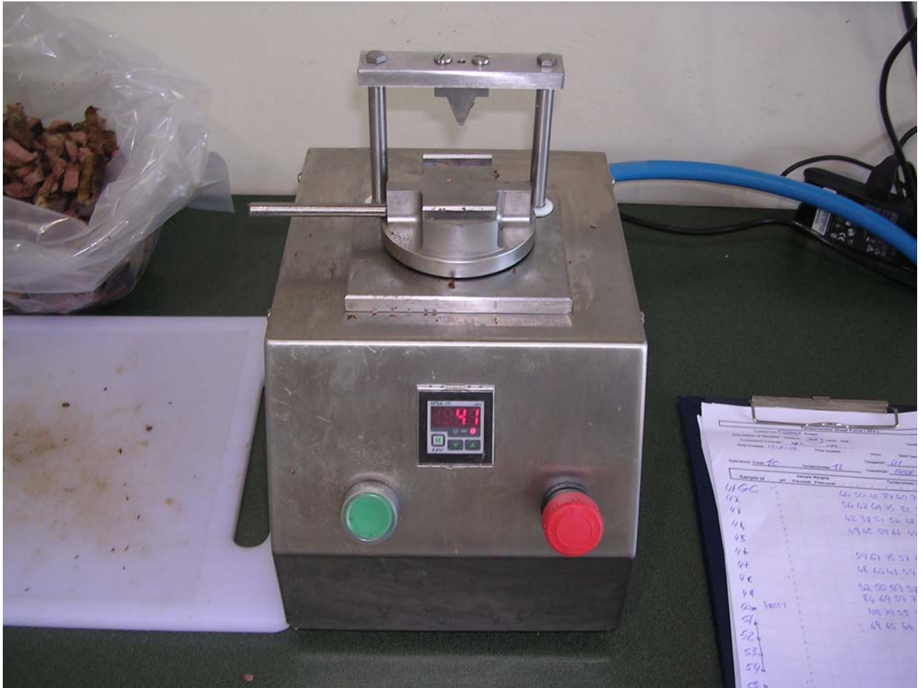
Figure 8. G1 Tenderometer apparatus includes a primitive display of the maximum pressure required to penetrate a cooked meat sample. A v-shaped blade is forced to penetrate the meat sample which is loaded into the fitted cavity.
